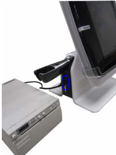
Figure 3-30 Connect B/W printer
