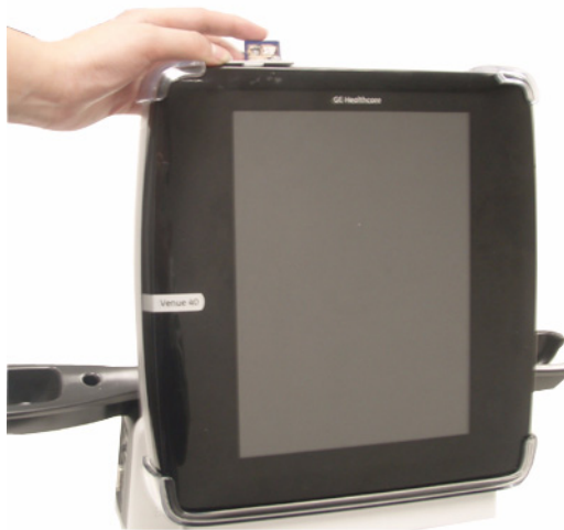
Figure 3-29 Insert SD Card to system
