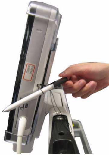
Figure 3-20 Thread the loop
