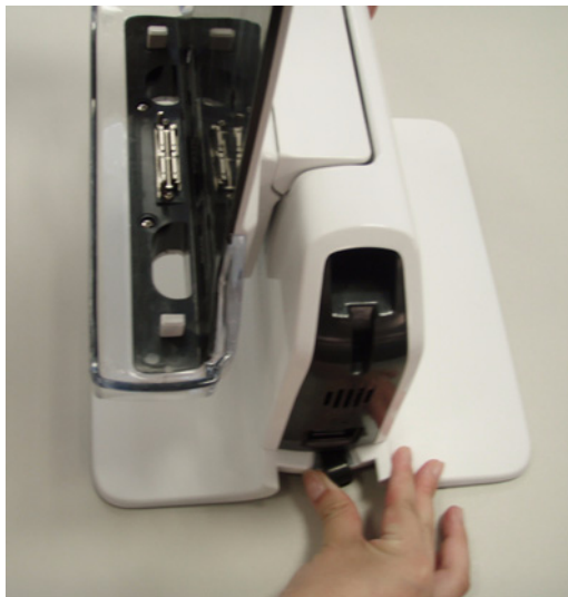
Figure 8-1 Docking Station Desk Support Assy disassembly
