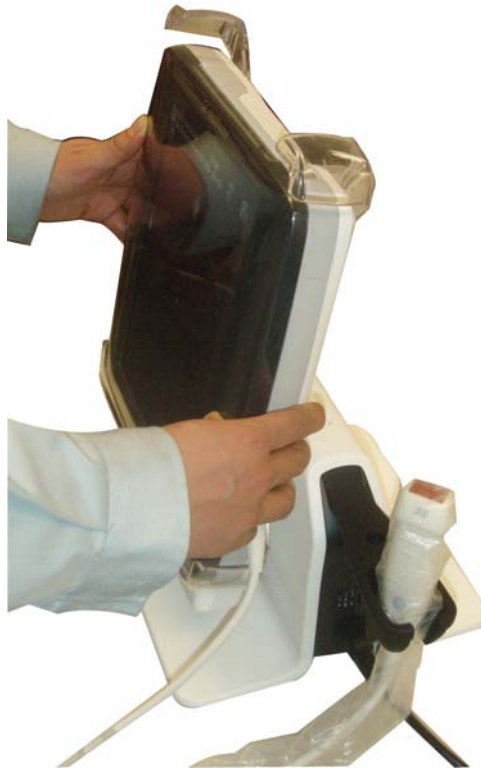
Figure 3-14 Mount system onto Docking Station/Docking Cart
