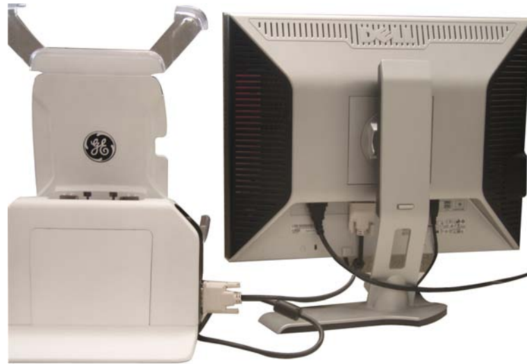
Figure 3-32 Connect external LCD
