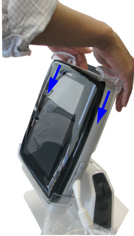
Figure 3-15 Press the locking lever
