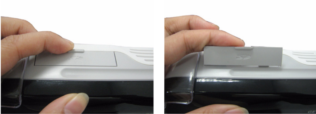
Figure 3-28 Open SD Card Socket cover
