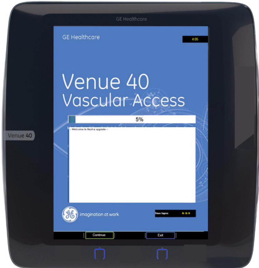
Figure 8-16 Upgrading process paused
