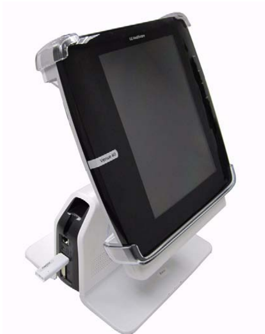
Figure 3-33 Connect the Wireless Network Card
