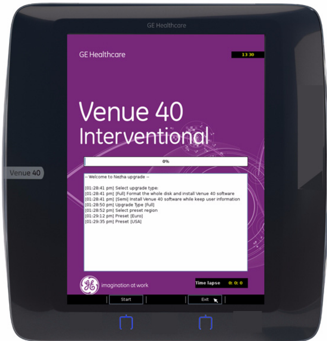
Figure 8-14 Startup screen for upgrading process
