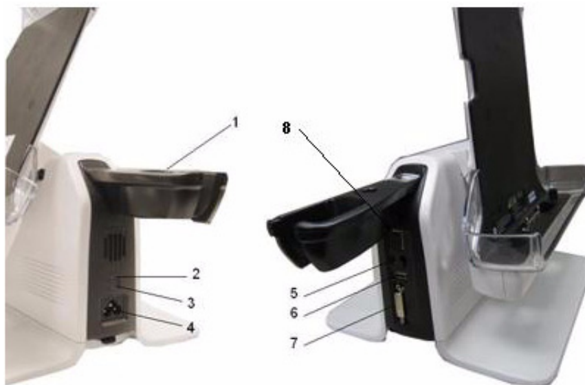
Figure 3-27 Docking Station/Docking Cart Connector Panel
