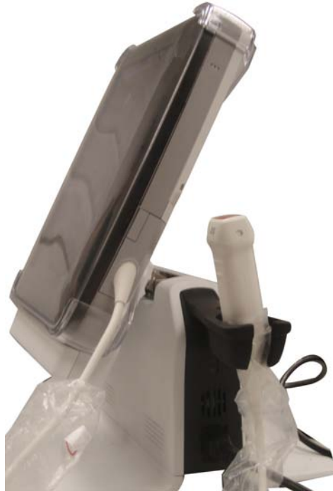
Figure 6-8 Tilt the LCD monitor
